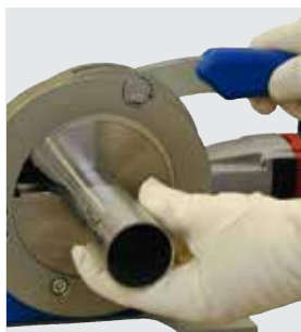
Quick clamping system for tools, clamping shells and tubes
