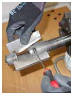
Fast adjustment of the pipe dimension
